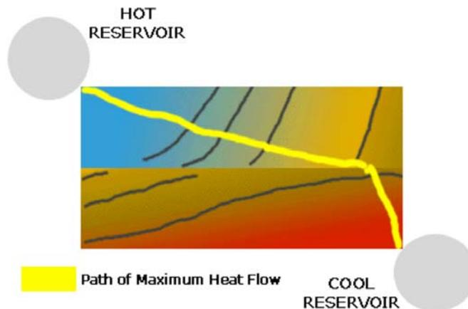
**FIGURE 3** Heat conductors in series with isotherms
